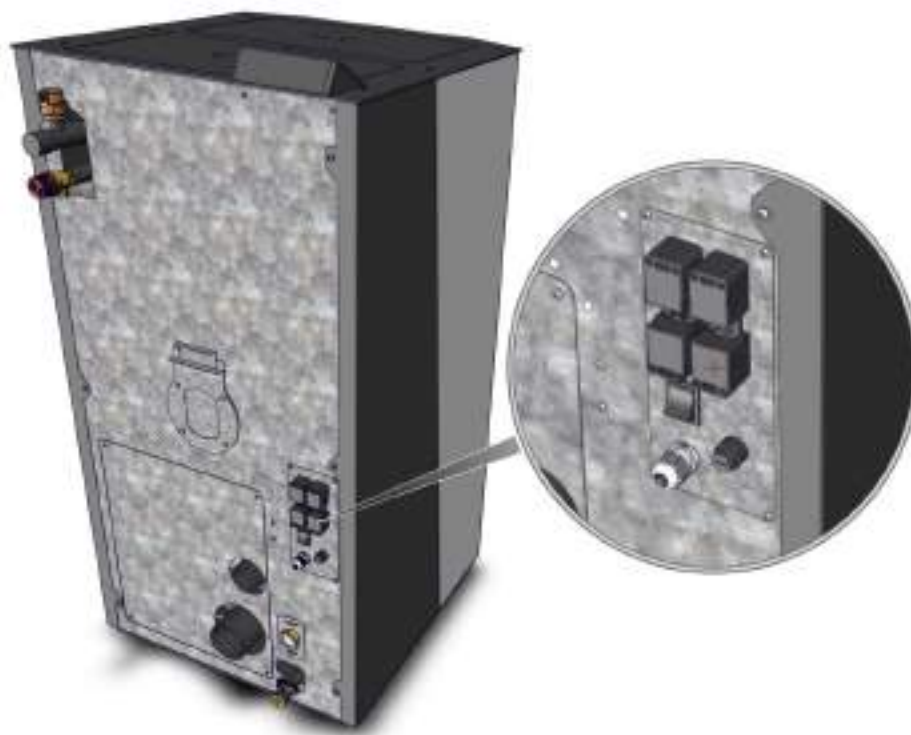
Picture 26. The positional representation of the cable grommet, main switch as well as the safety thermostat
