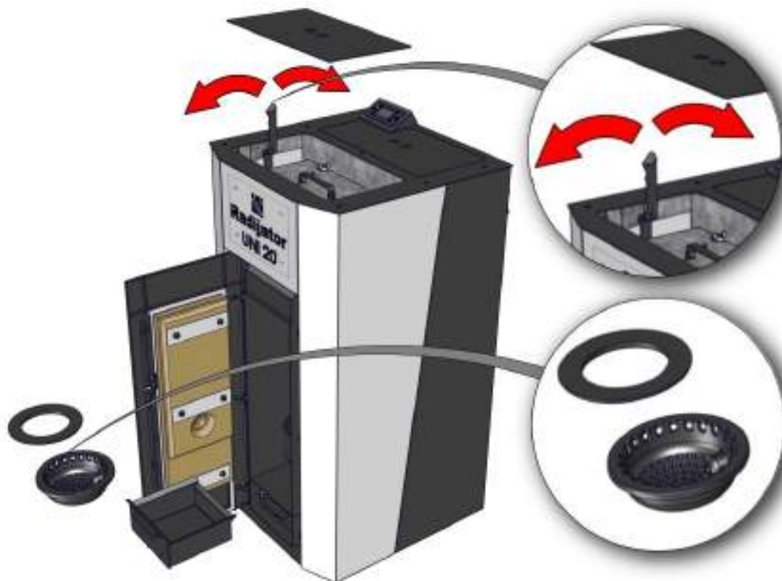
Picture 28. Cleaning the combustion cup and turbulator
