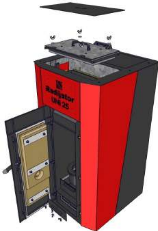
Picture 29. The representation of elements being disassembled during cleaning
