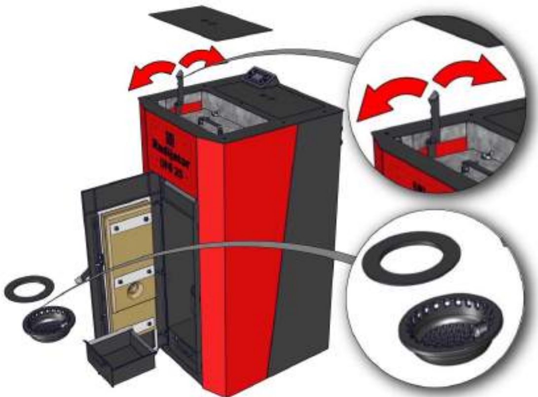
Picture 28. Cleaning the combustion cup and turbulator
